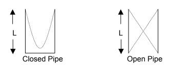
One closed pipe and one open pipe both the same length 'L' are taken for consideration. Formation of fundamental tone in both cases are shown in the 'above fig'. For closed pipe frequency of the fundamental tone is given by,
