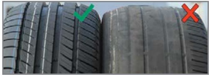
Figure 5.10 An example of a new tire and worn off tire
